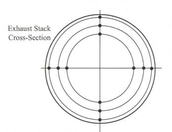
Velocity sample locations as measured from stack wall (not including 1.5" sampling port nipple)
