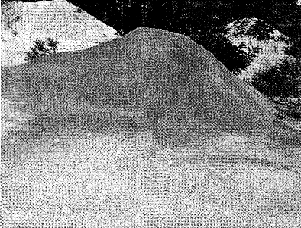
Image 4(crushed granite) : crushed granite pile near batch mixing
