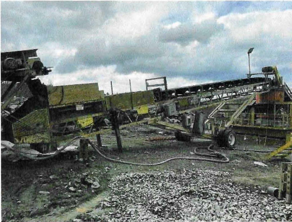
Image 5(Tilden5) : RS-28 Radial Stacker
