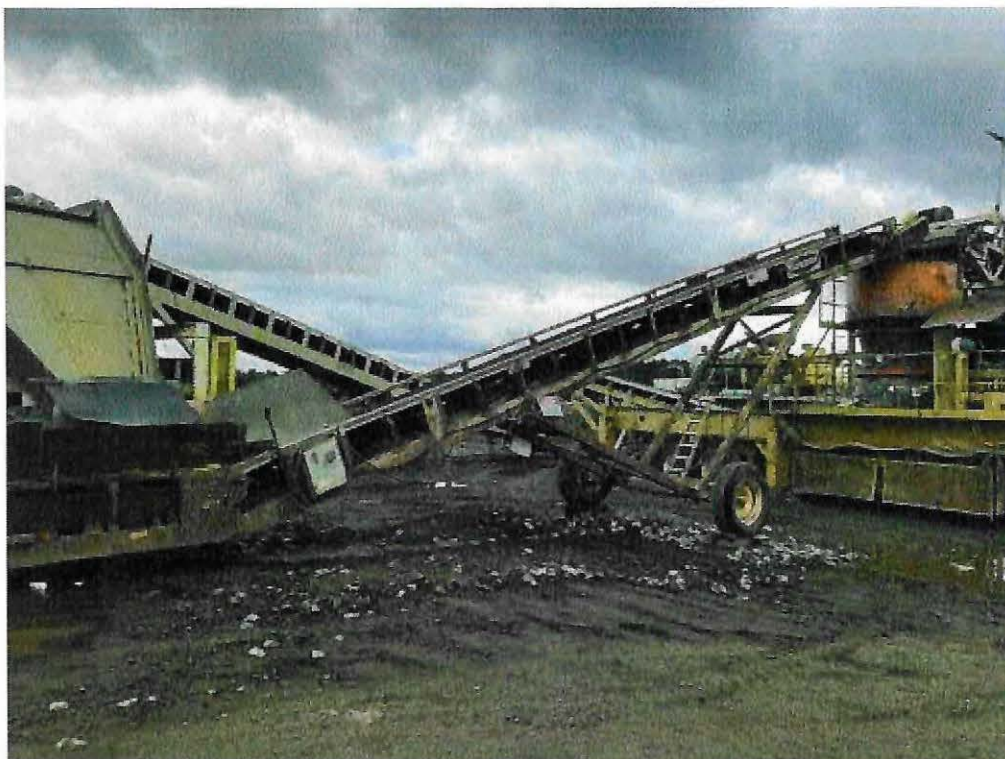
Image 3(Tilden3) : RS-11 Radial Stacker
