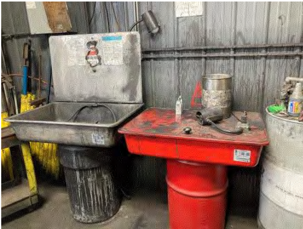
Image 3(Parts Washers) : Aqueous- (left) and Solvent-based (right) parts washers
