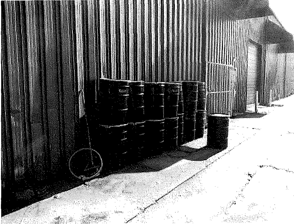
Image 4(Waste containers) : These currently empty drums are used to collect the magnesium and iron particles. They are sealed and removed once filled.
