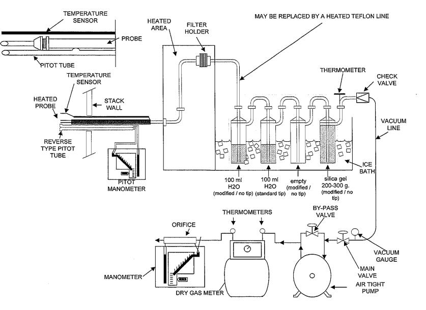
Figure 4.1 - EPA Method 4 Sampling Train Schematic
