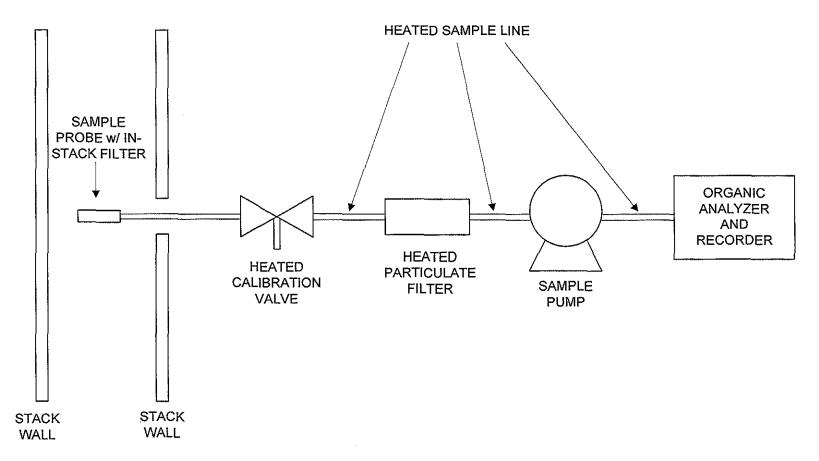
Figure 4.2 - EPA Method 25A Sampling Train Schematic
