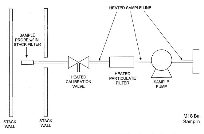
Figure 4.2 - EPA Method 18 and 25A Sampling Train Schematic
