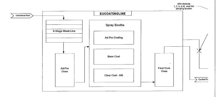
Figure 3.1 - EUCOATINGLINE Process Schematic
