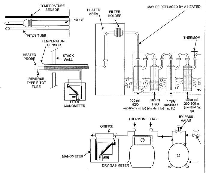
Figure 4.1 - EPA Method 4 Sampling Train Schematic
