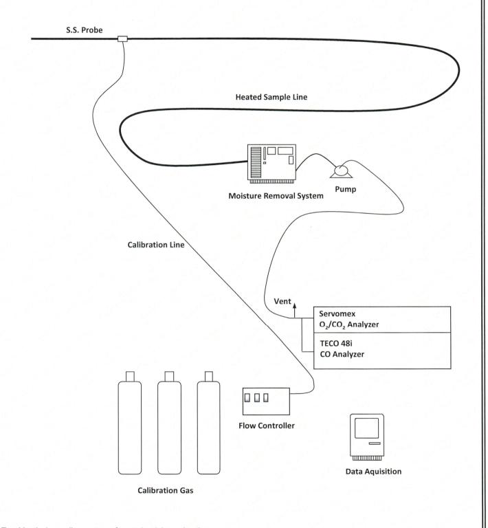
Two identical sampling systems for catalyst inlet and outlet.
