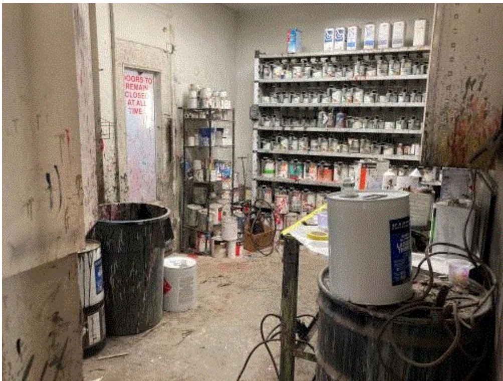
Image 3(IMG_0218.JPG) : May 14, 2021, The paint mixing room with multiple sources of uncontrolled fugitive
