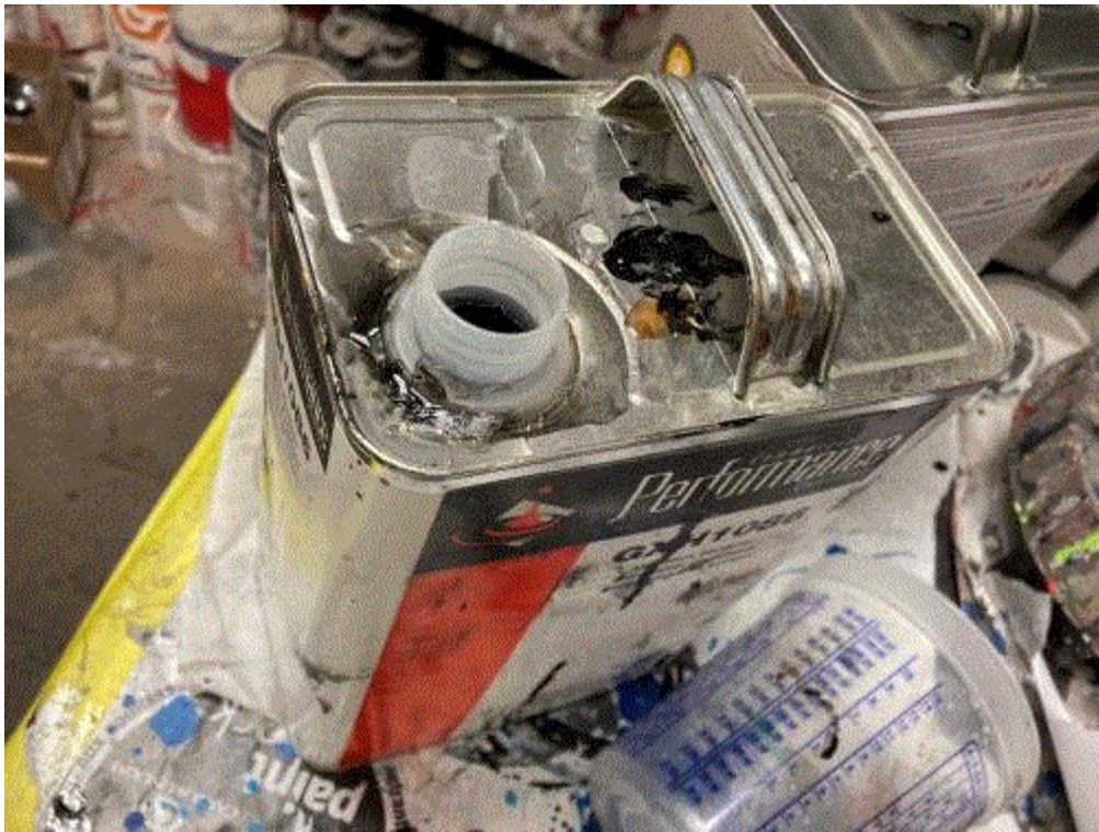
Image 5(IMG_0222.JPG) : May 14, 2021, uncovered can of solvent thinner that was one of the sources of fugitive emissions in the paint mixing room.
