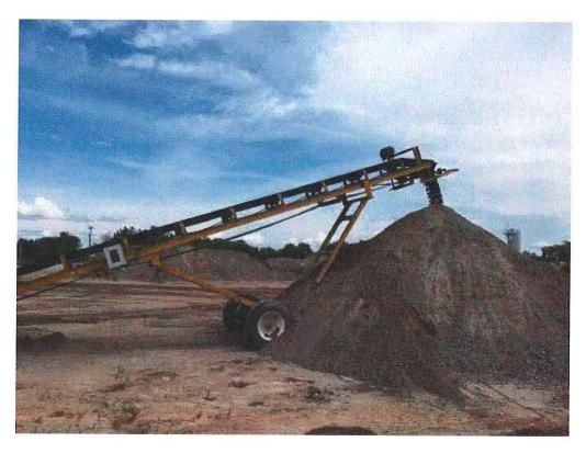
Image 7(Stacking Conveyor): Stacking conveyor with belt scale. No visible emissions observed from storage piles.
