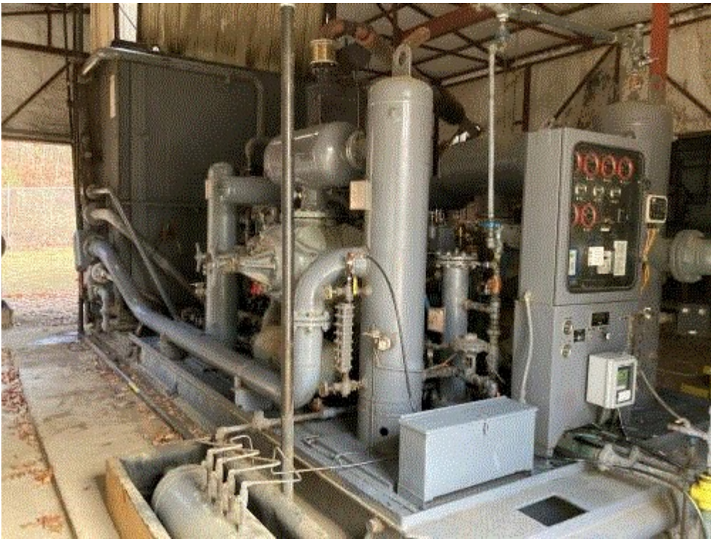
Image 2(EUENGINE) : Engine on site. Skid #104453, 948RPM, 45 PSI, 302 Deg F
