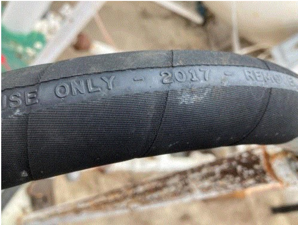
Image 13(Hose Date) : 2017 manufacture date on one of the permanent storage tank hoses.
