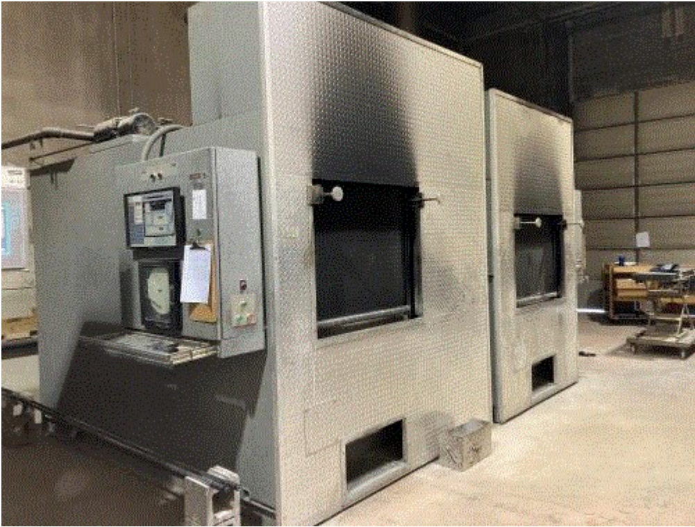
Image 1(IMG_0293.JPG) : Cremation units EUCREMATORY5 and EUCREMATORY3 (left to right). This photo was taken to document the soot deposits on the exterior of each machine. All cremation units had similar soot deposits.
