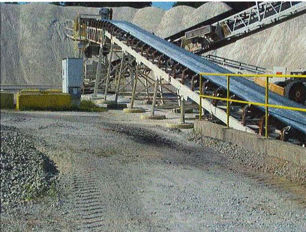
**Image 7(Residual Coal #2)** : Darker area by conveyor is residual coal from past coal handling activities
