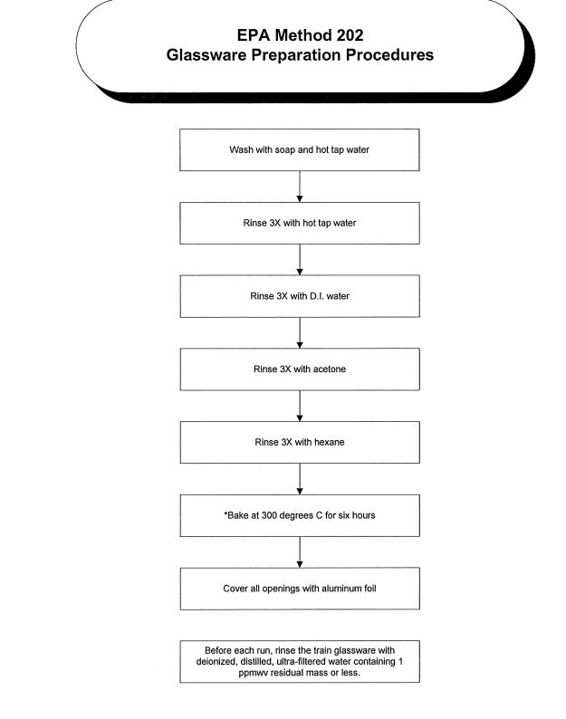
\*As an alternative to baking glassware, a field train proof blank can be performed on the sampling train glassware.
