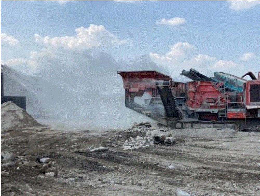
Image 4(4) : Heavy opacity from Terex Finlay feeder (TF) and portable crusher (TC) just before shutdown.
