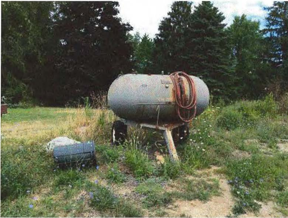
Image 5(190) : Calcium chloride tank
