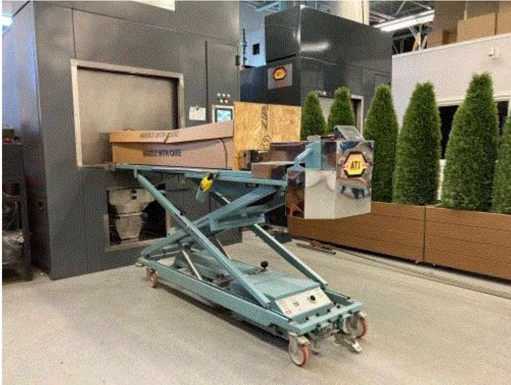
Image 3(IMG_0191.JPG) : Lift table with scale and ram. Note: the lift table must be set to lowest position to measure the charge weight. To conceal personal information, a piece of wood was placed between the charge and ram. The wood is not required for normal operation.
