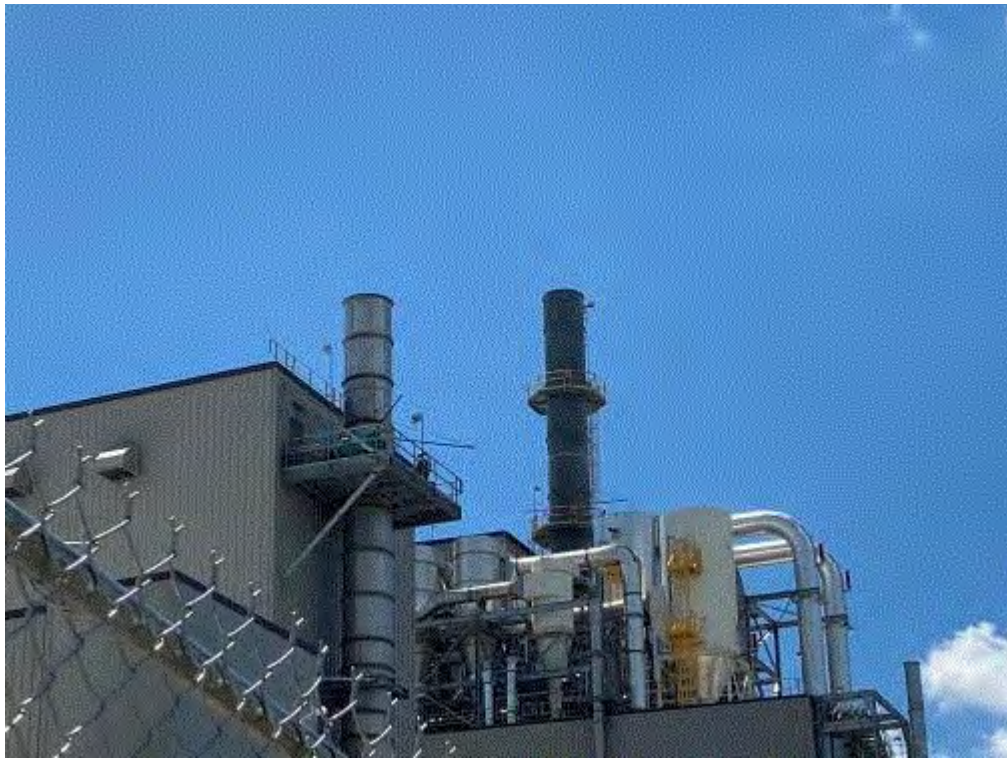
Image 1(SVDC - SVPREP) : Gray stack is SVPREP, silver stack is SVDC. No opacity, taken during stack test of these units.
