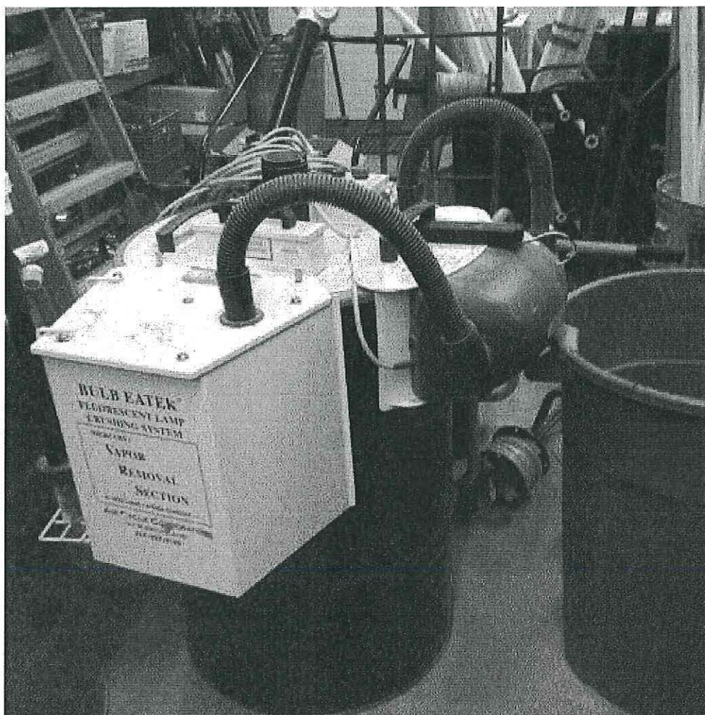
Image 2(Bulb crusher) : Code Electrical bulb crusher, photo taken on February 17, 2016.
