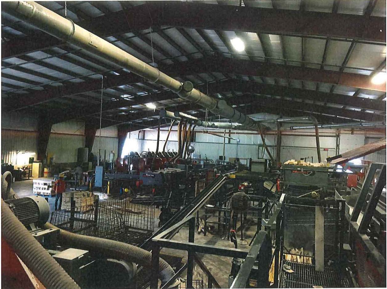
Image (1): Sawdust is collected at generation points and pneumatically conveyed to the baghouse.
