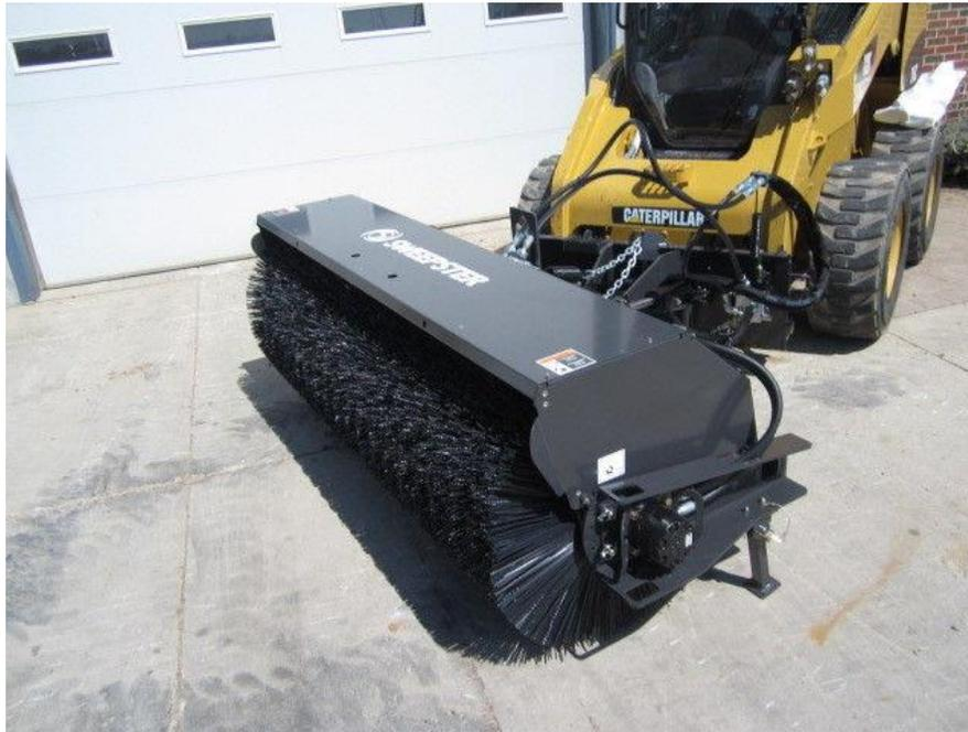
FRC yard is swept as needed with a sweepster power broom attached to a CAT 242b skid steer very similar to the one pictured above. The yard is only swept after it has rained or been watered down to minimize dust.
