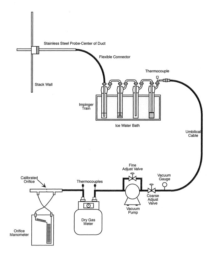
Figure 3.2 USEPA Reference Method 4 sampling train
