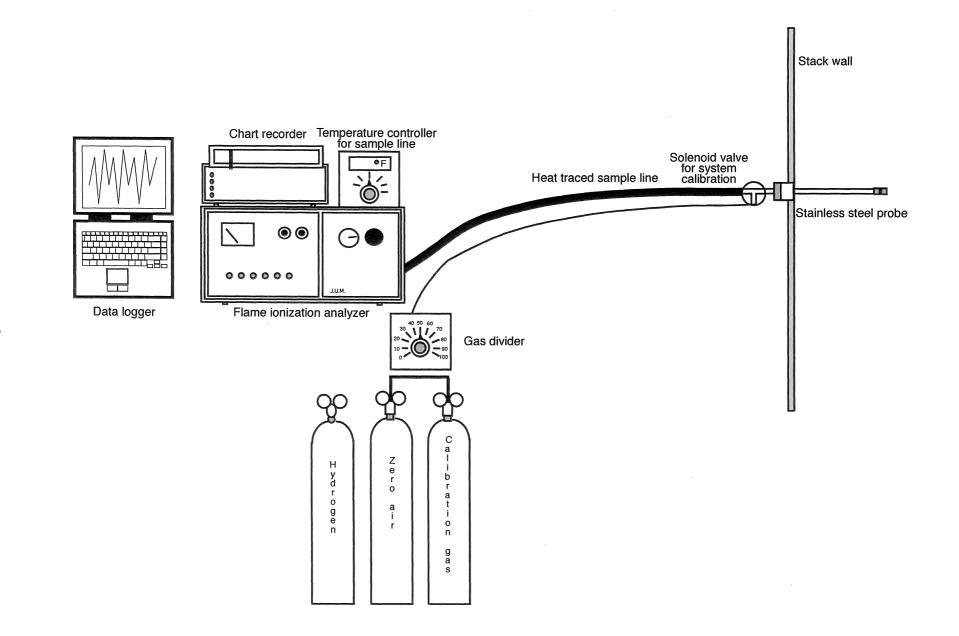
Figure 3.3 USEPA Reference Method 25A measurement system
