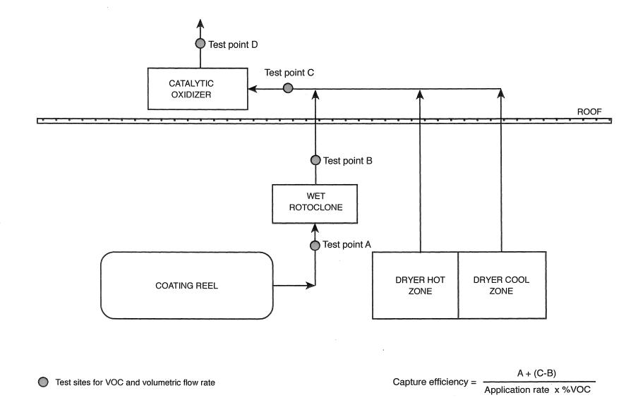
Figure 3.1 Process flow diagram
