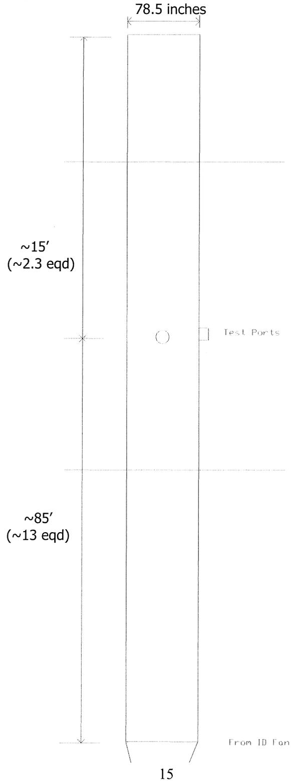
**Figure 5-2: Test Port Location (Outlet Ground Site)**
