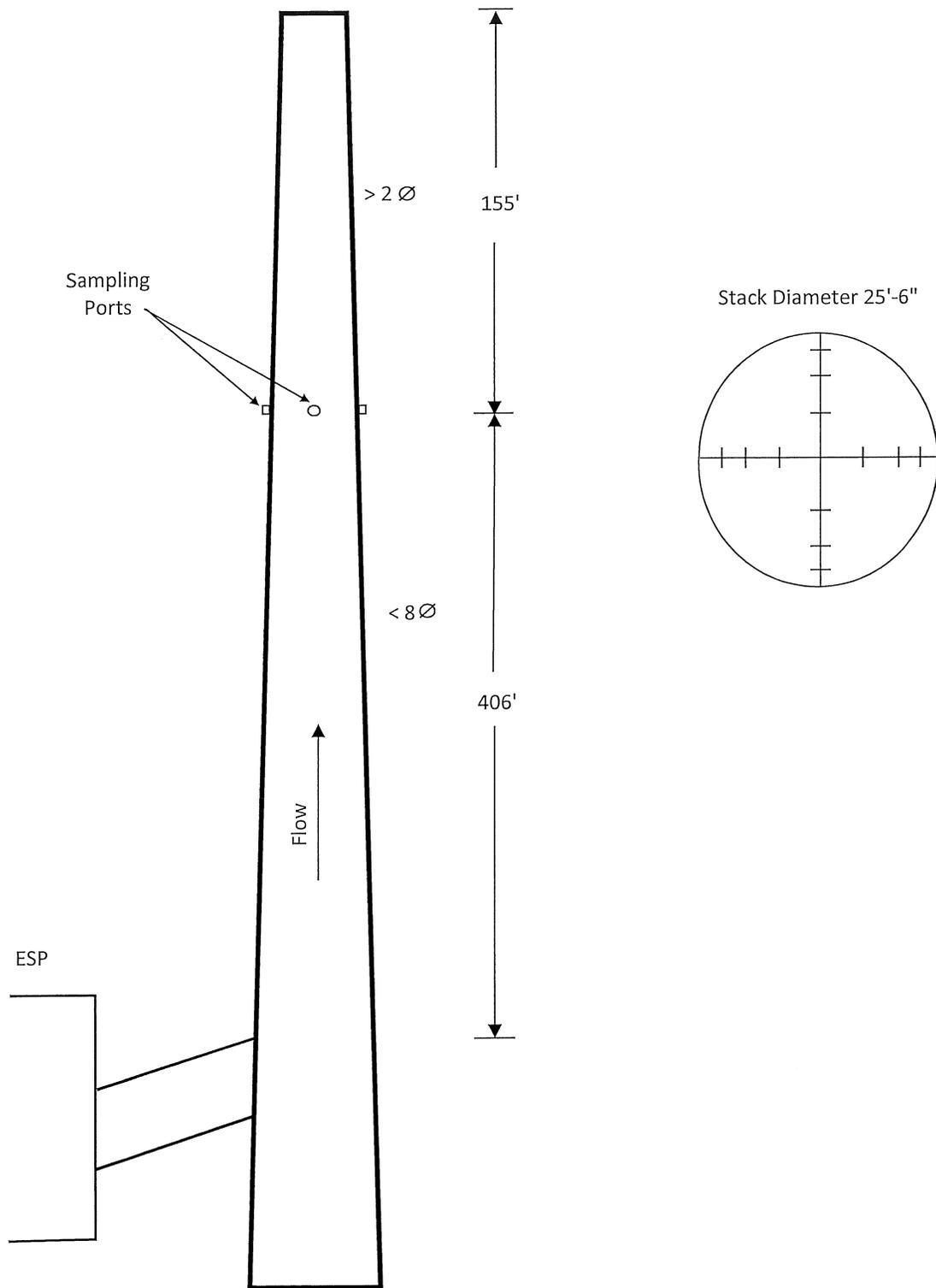
Figure 2 – ASTM D6348
