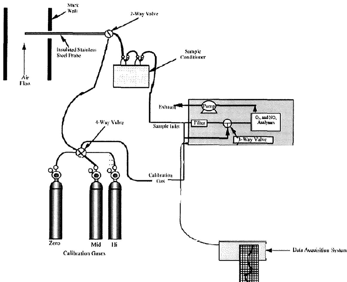
**Figure 4-2. USEPA Methods 7E and 10 Sampling Train**
