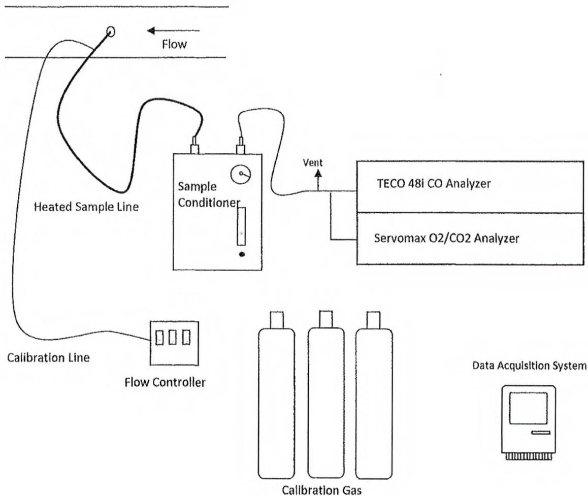
**Figure 3 – ASTM D6348/ 3A
