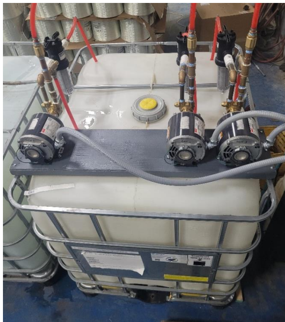
Figure 12. Ecosorb batching and pumping totes plus system.
