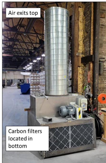
Figure 11. Carbon Filter and Ecosorb distribution recirculation towers
