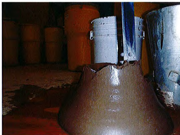
Figure 18: Left: 7" Slump, Right: 10" Slump
