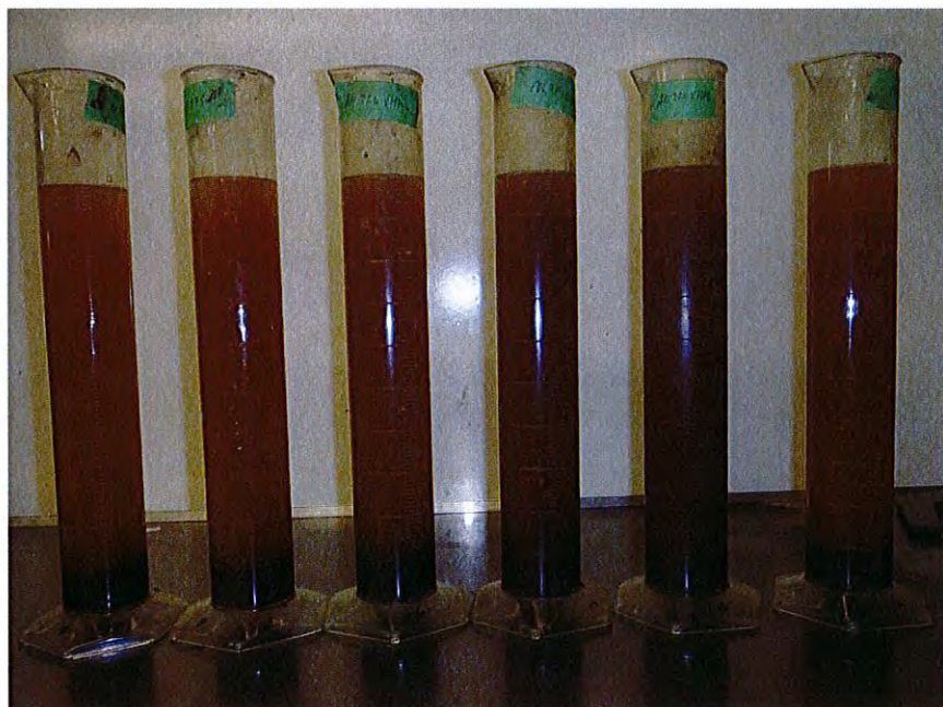
Figure 8: Flocculant Screening Cylinders
